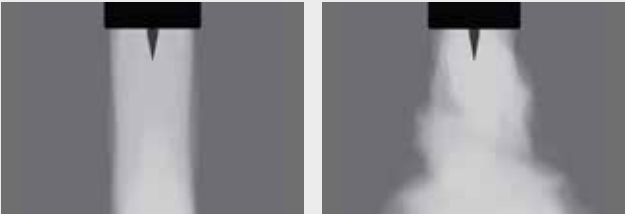
The picture on the right shows a highly turbulent flow, offering poor shielding and elevated gas consumption.
